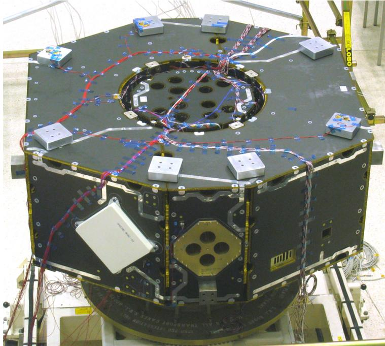
**Figure 11:** LISA Pathfinder flight structure being prepared for the first of the environmental test campaigns.
