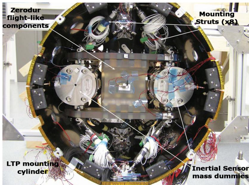
**Figure 18:** Photograph of the LISA Technology Package Core Assembly (LCA) in preparation for vibration testing.
