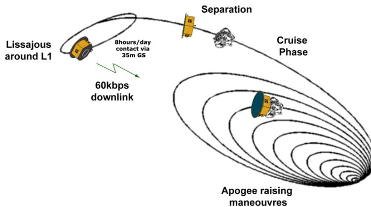
**Figure 4:** Schematic of the LISA Pathfinder orbit from launch to science operational orbit.
