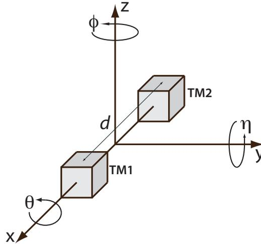
**Figure 12:** LTP Test Masses layout schematic and axis rotation angles notation
