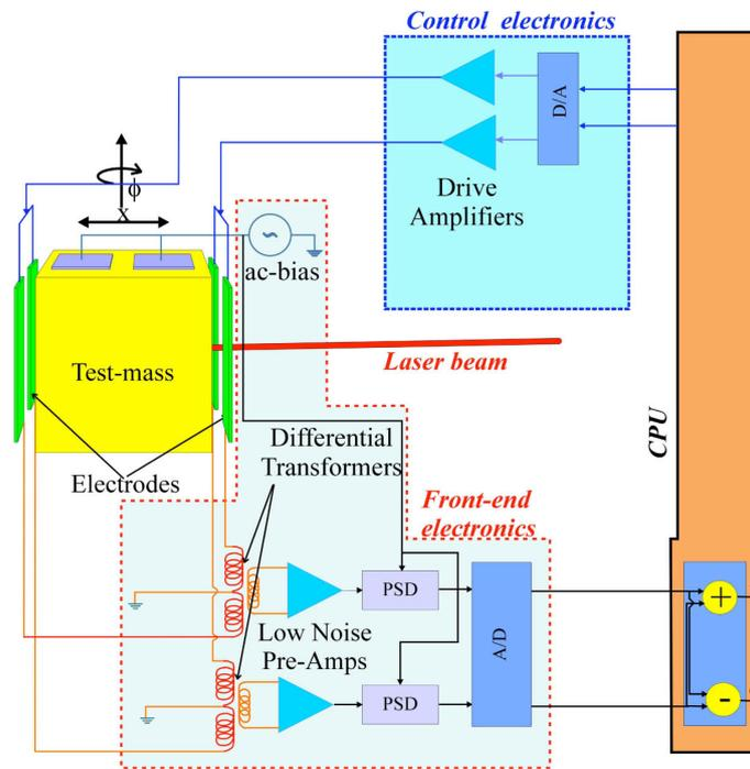
**Figure 8:** Schematic diagram of the operation of the inertial sensor capacitive readout and actuation electronics.
