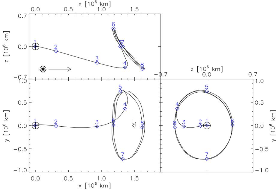
**Figure 3:** Reference trajectory for LISA Pathfinder. The trajectory is shown in synodic (co-rotating) frame with the Earth at the origin, the x-axis pointing into the Sun direction, and the x-y plane being the plane of the ecliptic. The z-axis (out-of-plane axis) is chosen to form a right-handed coordinate system. The markers show the positions of the spacecraft at different epochs.
