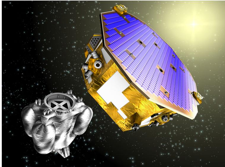
**Figure 5:** Artist impression of LISA Pathfinder after separation of the science module from the propulsion module before reaching the operational orbit around L1
