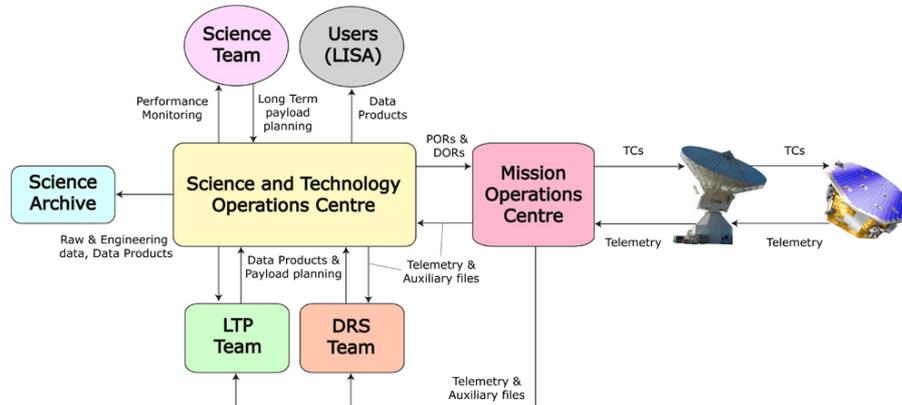
**Figure 15:** Overview of the LISA Pathfinder Ground Segment diagram showing the data flow.
