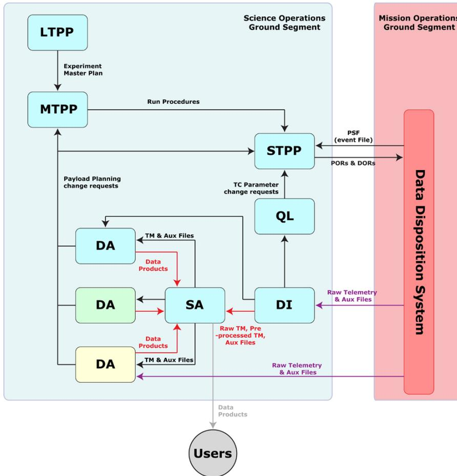
**Figure 16:** Overview of the science operations ground segment showing the data flow between the various subsystems.
