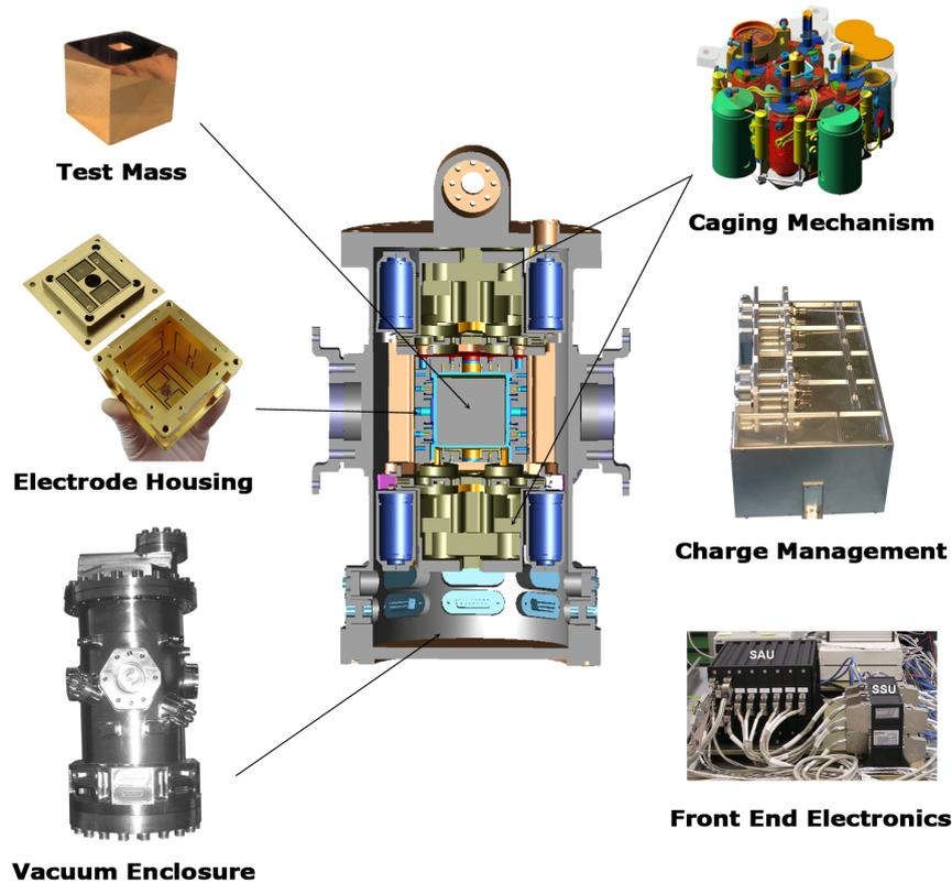
**Figure 9:** The Inertial Sensor. The centre graphic shows a cut-away of the Inertial sensor vacuum enclosure. The photographs around the side show engineering models of the ISS subsystems (with the exception of the drawing of the caging mechanism which is shown for clarity)
