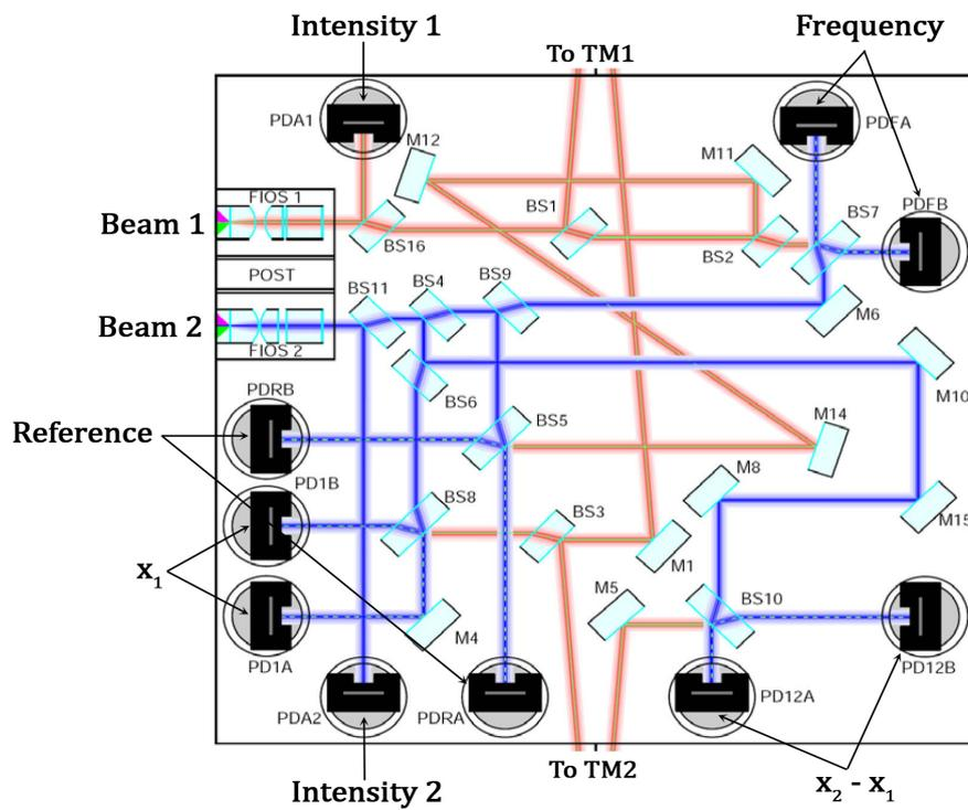
**Figure 10:** Optical Bench Interferometer layout. The labels *To TM1* and *To TM2* indicate the positions of the test masses (not shown).
