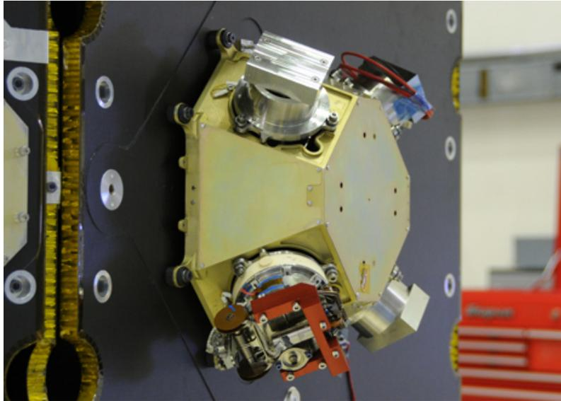
**Figure 14:** Engineering Model of the Slit FEEP Cluster Assembly mounted on the spacecraft during the acoustic test at system level. The cluster shown consists of one FEEP thruster EQM (bottom) and three mass dummies. The four thrusters are in the launch configuration of lids closed. A lid opening mechanism is operated before the thrusters can be used in orbit.
