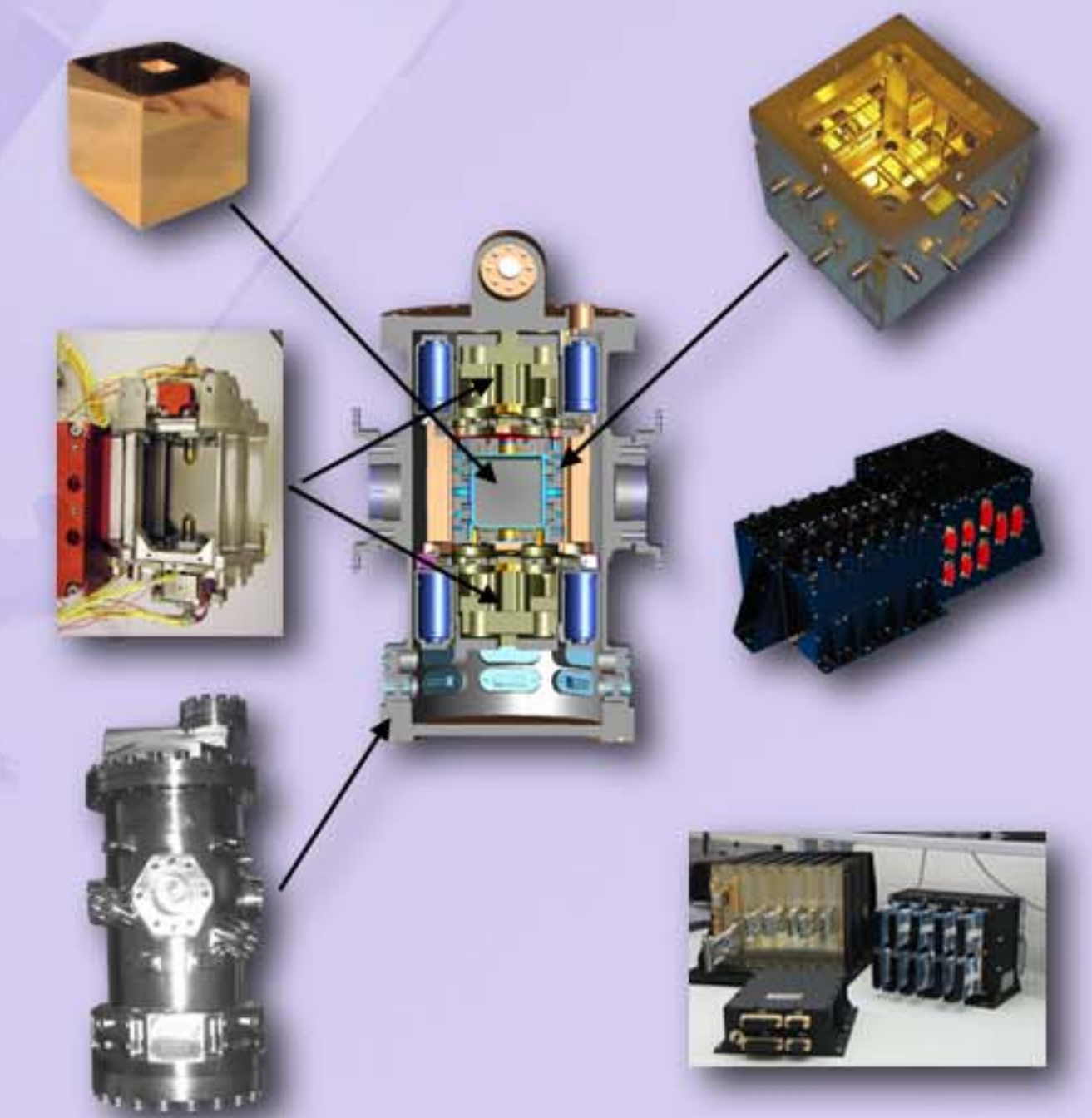
Photographs of the Inertial Sensor Subsystem units. From top left (clockwise): Au:Pt test mass, electrode housing, UV lamp unit, front-end electronics, Ti vacuum chamber, caging mechanism
